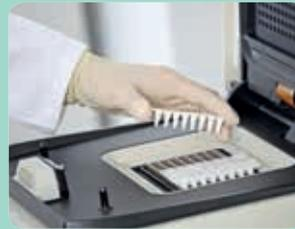
Place the PCR plate in the real-time cyclor and run the PCR program.
